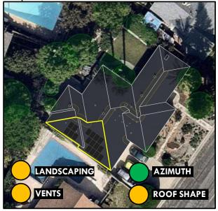
Example of optimal azimuth with optimal vent location avoiding the solar optimal roof face.
