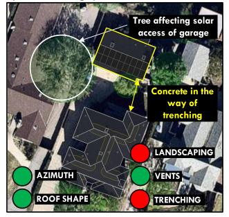
Example of detached structure with optimal azimuth and an optimal trenching option for conduit.
