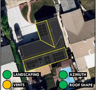
• If the home has a detached garage it may be a good candidate for all or part of the homes solar system. Uninhabitable structures like garages and carports do not need the same fire setbacks as a home, so more solar modules can be placed on the same amount of roof area on a garage as on a home.
